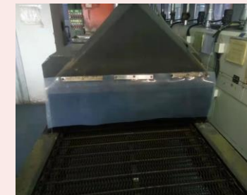
Replacing the draft shield of the tunnel furnace
